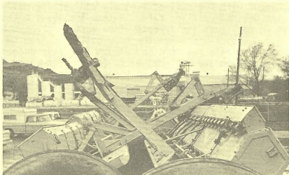
Figure 23. Drills should be loaded with tongues offset and crossed, pointing towards each other.
